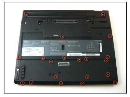
Using a Phillips #0 screwdriver, identify and unscrew the twenty screws located on the underside of the T42.
