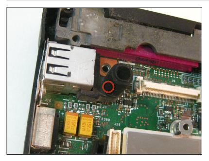
Remove the rubber cover from the microphone.
