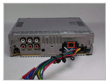
Locate the clip on the wiring harness.
