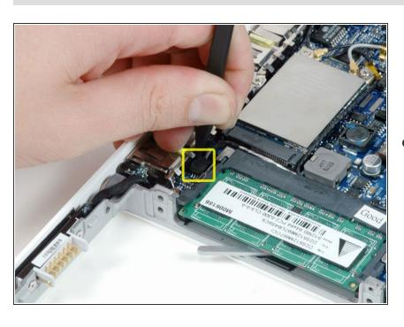
Use a spudger to carefully disconnect the microphone cable from the logic board. You'll want to
