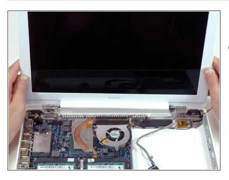
Grasp the display assembly on either side, and lift it up and out of the computer. To reassemble your device, follow these instructions in reverse order.
