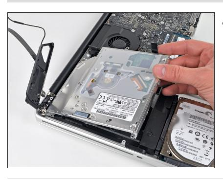
Lift the optical drive near its connector and pull it away from the upper case to remove it from the computer.
