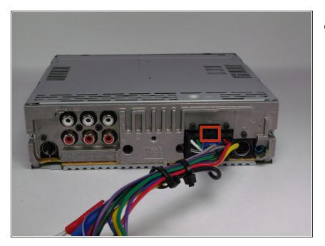
Locate the clip on the wiring harness.
