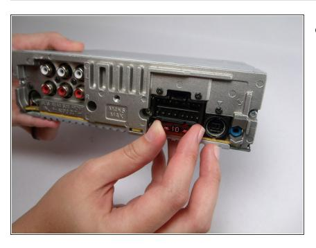
Using your index finger and thumb on either side of the fuse.
