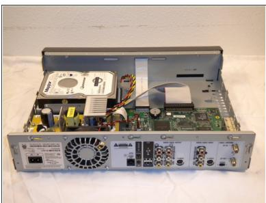
Lift up and pull back the outer casing towards the rear of the unit.
