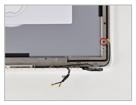
Remove the single 3.3 mm Phillips screw securing the lower antenna ground strap to the rear display bezel.
