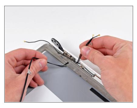
Carefully pull the antenna cables out from under the frame attached to the rear display bezel and remove them from the display assembly.
