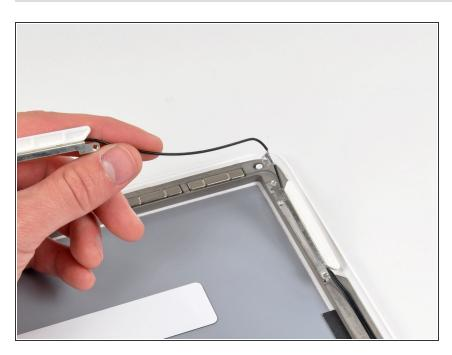
De-route the antenna cables from the slot cut into the rear display bezel.
