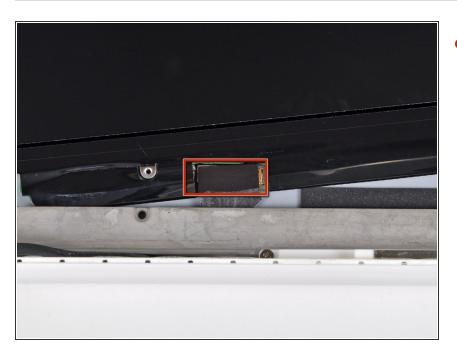
Peel the piece of tape covering the display data cable connector away from the edge closest to the LCD.
