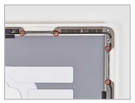
Remove the four 2.3 mm Phillips screws securing the two antennas to the rear display bezel.
