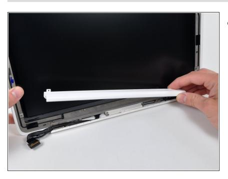
Remove the clutch cover from the display assembly.
