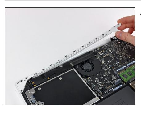
Carefully lift the rear vent out of the upper case.
