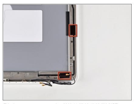
Remove the two small pieces of black tape securing the antenna cables to the rear display bezel.
