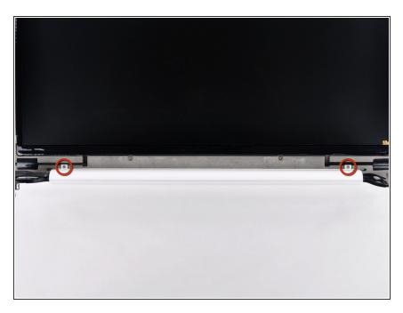
Remove the two 3 mm Phillips screws securing the clutch cover to the rear display bezel.
