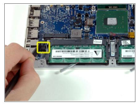
Use a spudger to carefully disconnect the microphone cable from the logic board. You'll want to work from side to side, and slowly wiggle the connector out of its socket.
