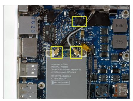
• Disconnect the two antenna cables from the Airport card, and the black inverter cable from the logic board.
