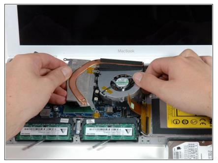
Hold the heat sink with one hand and the fan with your other hand, and lift the heat sink and fan assembly out of the computer. The fan is attached to the heat sink only with a strip of black felt tape, so be sure to remove both parts as a unit
