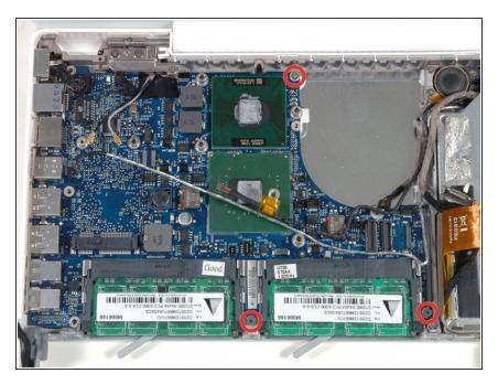
Remove the three 3 mm Phillips screws securing the logic board to the lower case.
