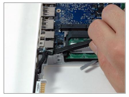
• Use a spudger to carefully pry the battery connector up and disconnect it from the logic board.
