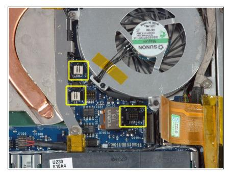
• Disconnect the black fan connector and two white temperature sensor connectors from the logic board.
