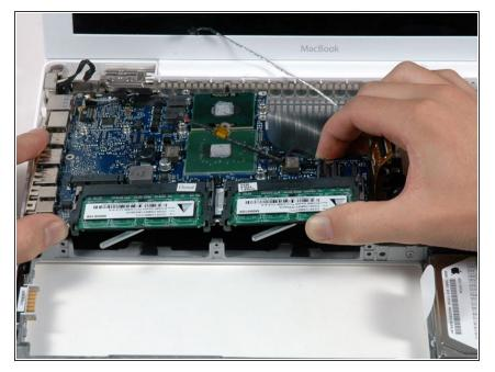
• Lift the logic board up from the right side, and slide it up and out of the computer.
