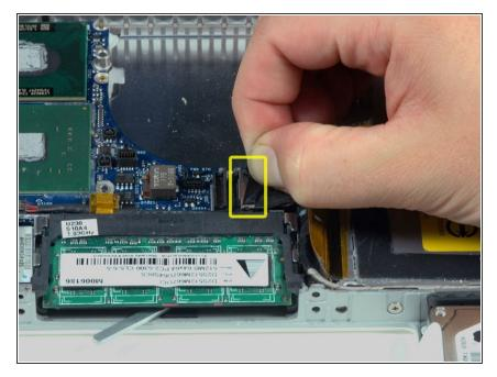
Disconnect the display data cable by pulling up on the black plastic pulltab. If there is no pull-tab on the top of the connector, it may be helpful to use a spudger to disconnect this connector.
