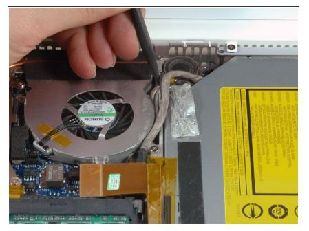
Use a spudger to move the gray display data and black speaker cables to the right. This will reveal a silver screw securing the fan housing to the lower case.
