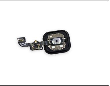
• We peel the home button off the front panel assembly with ease—though, as ever, the surrounding rubber gasket is easy to tear if you don't have the steady hands of a tech surgeon.
