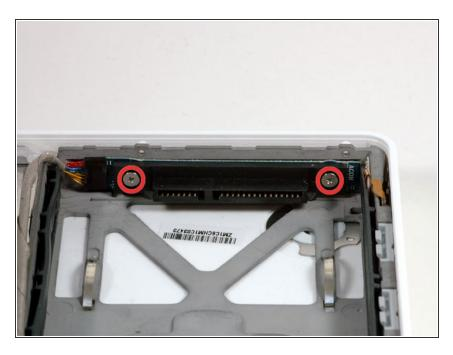
Remove the two Phillips screws securing the hard drive connector to the lower case.
