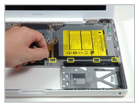
Deroute the hard drive connector cable from the four tabs along the edge of the optical drive.
