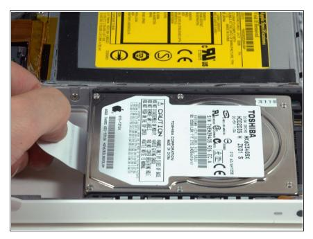
Use the white plastic pull-tab to slide the hard drive to the left and out of the computer.
