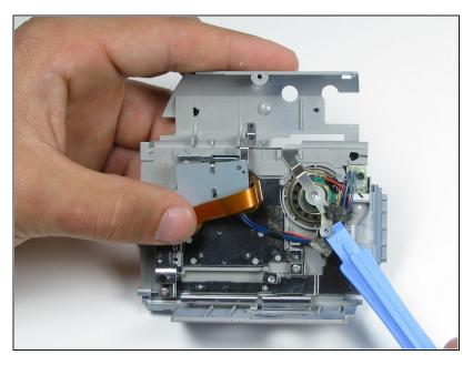
The speaker is soldered to both ends of the board. Check the connections to see if they are still good. Desolder wires from speaker to replace, if necessary.
