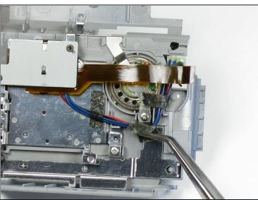
• Using tweezers, remove the black tape that is holding the speaker in place.
