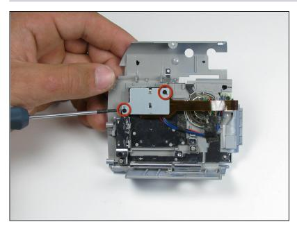
On the LCD housing plate, remove the two 4.5mm phillips screws on the ribbon cable plate using a #00 philips screwdriver.
