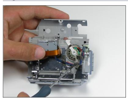
• Using #00 philips screwdriver, remove the 4.5mm silver screw on the speaker bracket.
