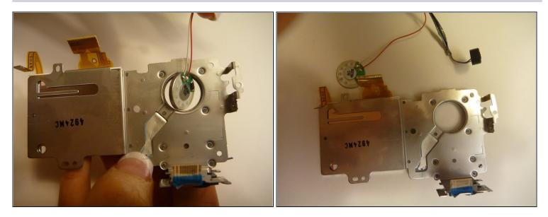
• Gently lift the speaker from the LCD screen fitting.
