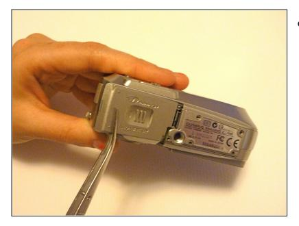
Press and slide the battery cover retainer clip to the left. Use <u>tweezers</u> to lift the battery cover away.
