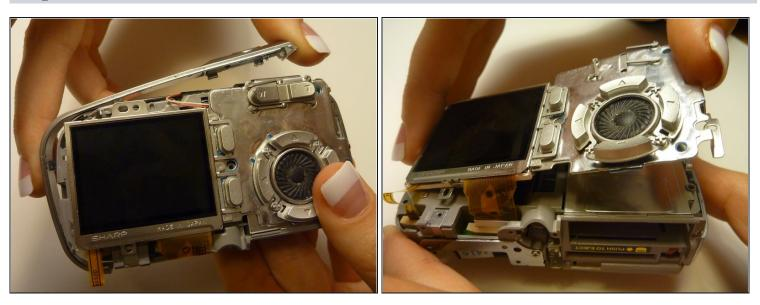
• To check that all screws are removed from the exterior side panel, gradually slide and lift no more than 3cm away from the camera internal component body.
