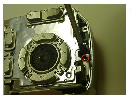
Remove one screw Phillips #00 from the right side of the LCD screen camera internal housing component.
