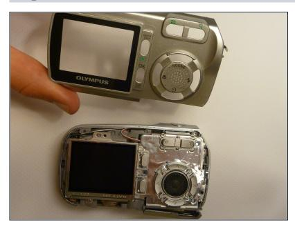
• Pull the backplate away from the camera internal housing component.
