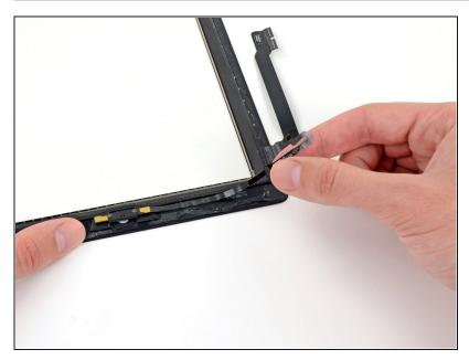
Carefully peel the home button ribbon cable from the front panel.
