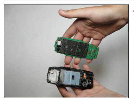
With the screws removed, the logic board can then be lifted out of the body by hand.
