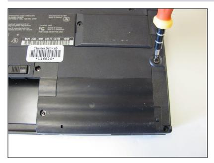
On the back of the computer, use a Flathead screwdriver to remove this lone screw.
