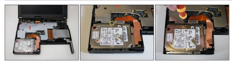
• Turn the computer back over so the hard drive faces up. Remove the shown screw with a Phillips screwdriver.
