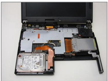
• Carefully lift and remove the keyboard.
