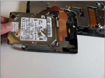
• Remove the final two screws (shown) and slide out the hard drive.
