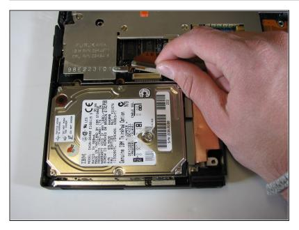
Make sure you are grounded and detach the IDA cable connecting the hard disk to the motherboard.
