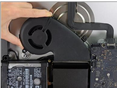
Lift and remove the fan from the iMac.
