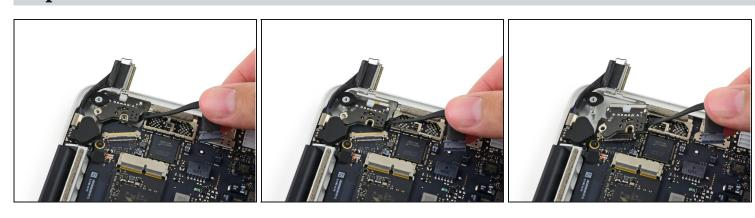
• Use the MagSafe DC-In board cable to pull the board out and up from the upper case to remove it.
