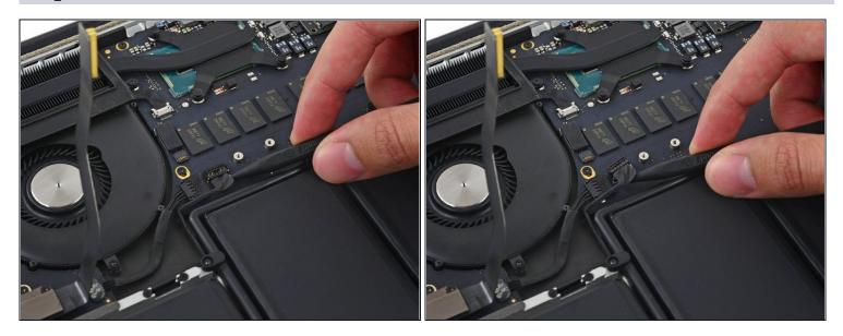
• Carefully tuck the tip of a spudger under the right speaker cable near the connector and lift it up out of its socket on the logic board.
