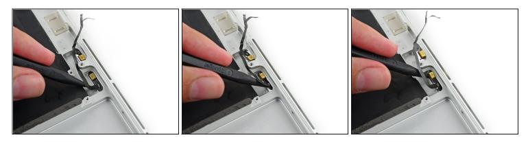
• Insert the tip of a spudger under the right-hand portion of the microphone ribbon cable and slide it toward the screw post to free it from the upper case.
