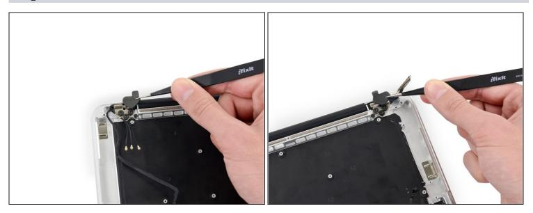
• Use a pair of tweezers to lift the rubber hinge covers up off the right and left display hinges.
