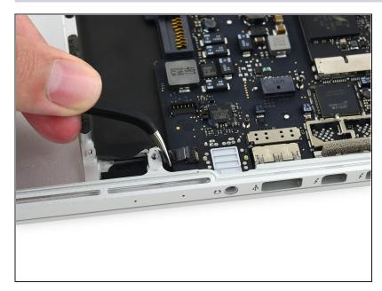
Pull the microphone cable straight out of its socket on the logic board.
