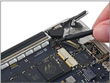
Use the flat end of a spudger to disconnect the keyboard backlight cable and move it out of the way.
