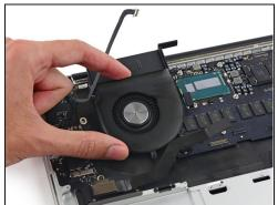
• Lift the end of the fan from the heat sink cavity and pull it up and out toward the hinge of the laptop to remove it.
