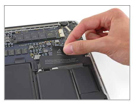
i If necessary, remove the plastic cover adhered to the battery contact board.
