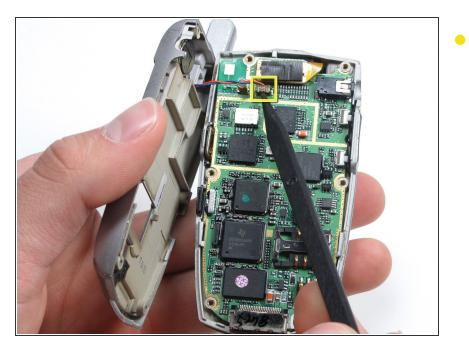
Use a spudger to disconnect antenna wire.
