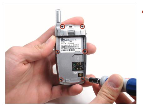
Use a T6 torx screwdriver to unscrew the 6 screws that hold the back casing on.
