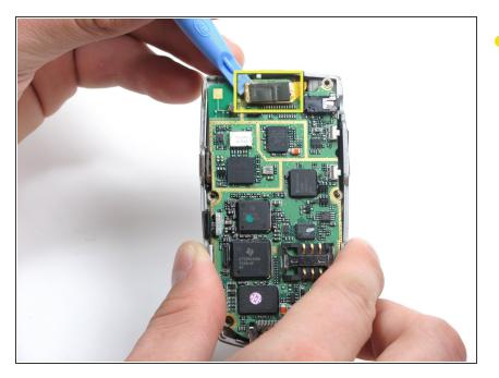
• Use the IPod opening tool to disconnect the main ribbon.
