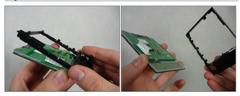
• The screen and internal frame should come apart easily. Set the screen on the cloth.
