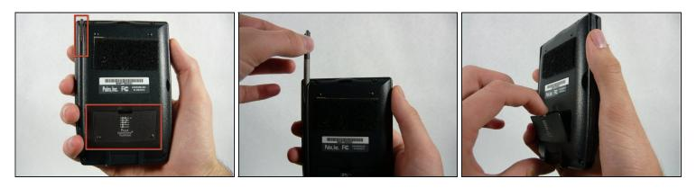
Turn the device over so it is face down and remove the stylus, and battery cover.
