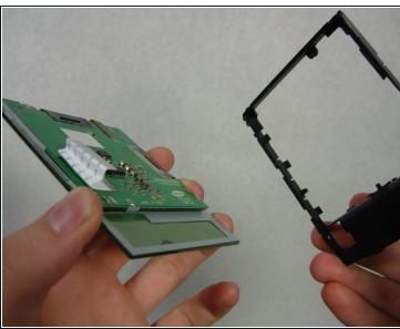
The screen and internal frame should come apart easily. Set the screen on the cloth.
