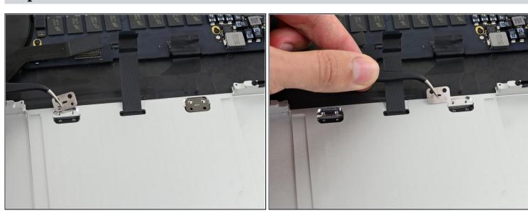
• Use <u>tweezers</u> to remove the two trackpad mounting brackets from the upper case.
