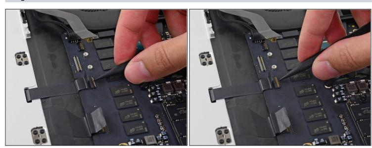
• Use the tip of a spudger to flip the retaining tab on the ZIF connector.
