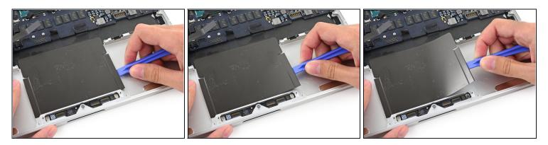
Use a plastic opening tool to slowly and carefully peel the trackpad cover plate up off the upper case.
