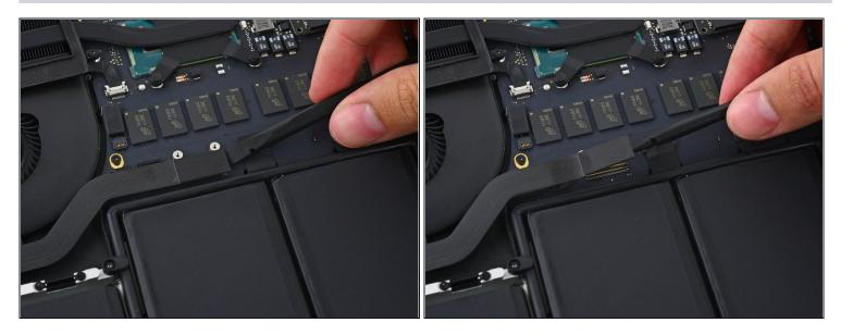
• Use the flat end of a spudger to pop the I/O board connector straight up off its socket on the logic board.
