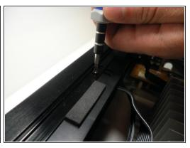
Unscrew the three screws on top of the face plate.
