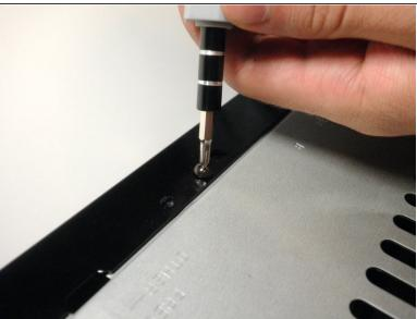
Unscrew the one screw on the bottom of the front panel.
