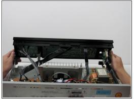
Simultaneously push down on the head of the snap on each end of the device with your thumbs and push to seperate the face plate. This may take some force.
