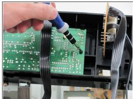
On the inside middle of the face plate you will see two screws in the logic board. Unscrew these two screws.
