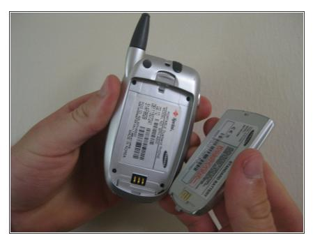
• Remove the battery from the phone, which will reveal four screws at the corners of the phone.
