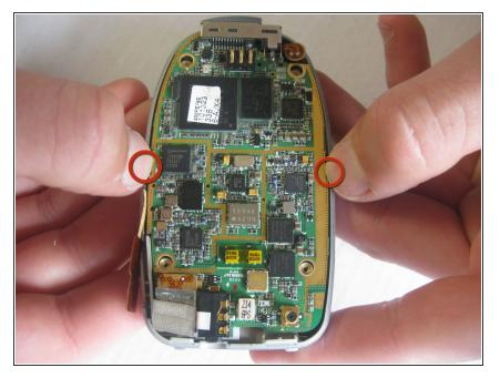
Pull the side tabs outward while simultaneously lifting up the circuit board.
