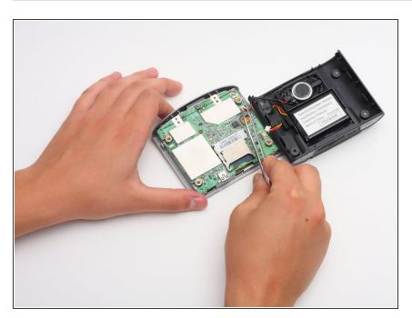
Once the two covers are separated, use the tweezers, or even your fingers, to gently disconnect the two sets of wires that are connected to the motherboard from the back cover. You may have to wiggle the wires a little bit to get them to disconnect.
