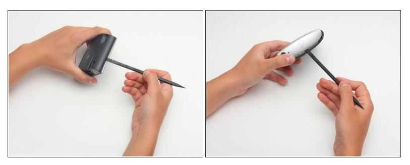
Using the spudger, gently pry apart the back case from the front case. It is easier to start on a side and work your way around the device.
