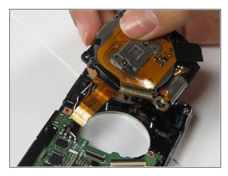
• Lift the lens unit free of the camera. A spudger can be used to separate the lens unit if necessary.
