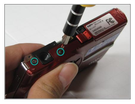
• Remove the two screws on the bottom of the front cover.
