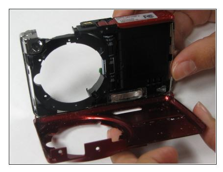
• Carefully lift off the front cover plate of the camera.
