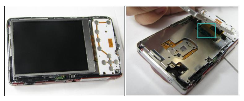
• Gently lift up on the left side of the LCD and slowly pull it to the left side of the camera but do not remove entirely, there is a ribbon connector.
