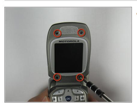
Unscrew the screws using a Phillips #00 Screwdriver.
