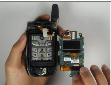
Remove the LCD board from the phone by grabbing the bottom side of the LCD board.
