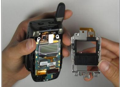
Place your thumb underneath the protective metal covering to remove it from the phone.
