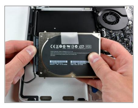
Lift the hard drive out of its supports and disconnect the SATA cable by pulling the connector straight away from the hard drive.
