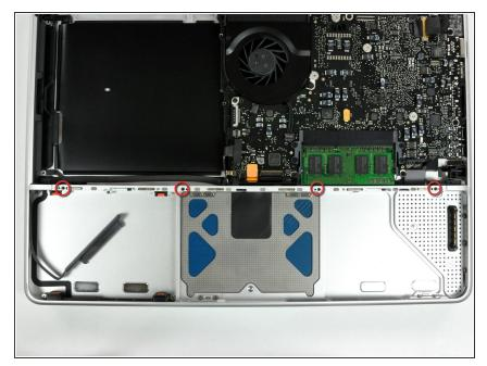
Remove the four 10.3 mm Phillips screws securing the mid wall to the upper case.
