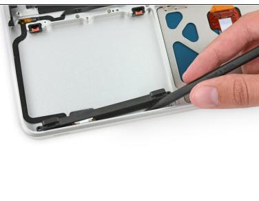
Insert the tip of a spudger between the hard drive bracket and the front edge of the upper case to free it from its recess.
