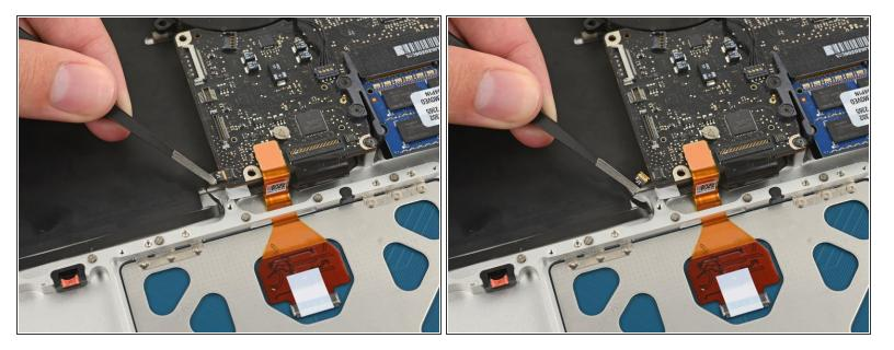
Pull the hard drive bracket cable out of its socket.
