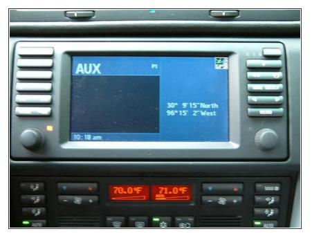
Once installed connect your audio device to the Aux Audio Input plug and use the MODE button to select AUX on your radio display
