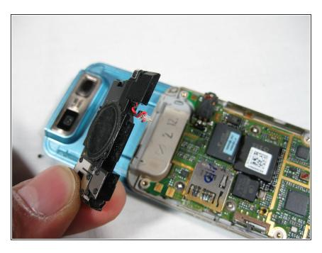
• Remove the speaker by lifting up.
