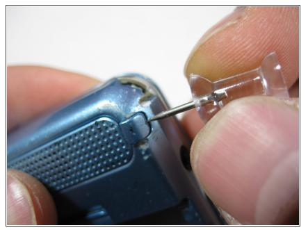
• Remove the 2 screw covers next to the rear speaker with a Push Pin.
