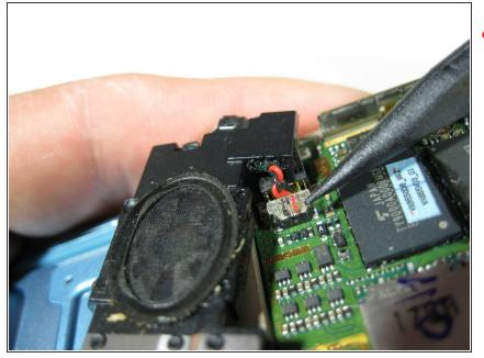
Carefully unplug speaker connector from circuit board with your fingers.
