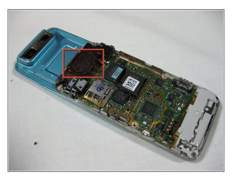
• With the back casing removed the speaker is visible.
