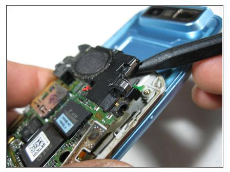
Lift up under top end of circuit board with the Spludger to access retaining clip.
