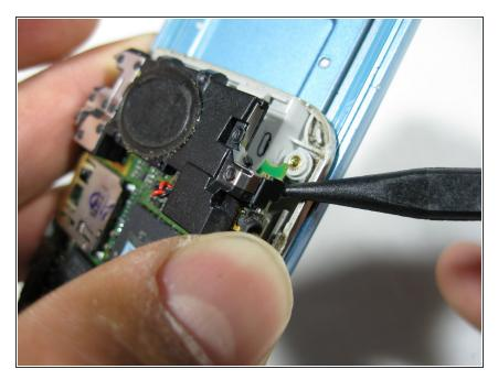
• Carefully pry up on retaining clip with the Spudger to release the speaker.
