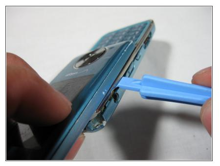
• Use the iPod opening tool to pry off the back casing.
