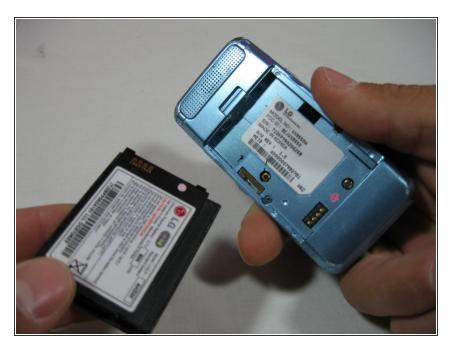
• Remove the battery by lifting away from the case.
