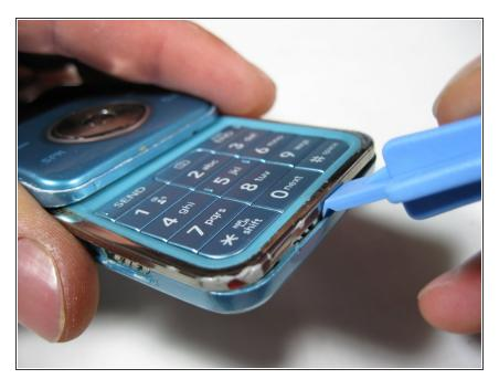
Continue sliding the iPod opening tool around the seam of the casing to separate the front and back casings.
