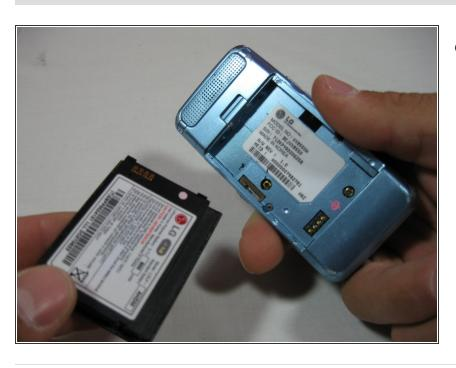
Remove the battery by lifting away from the case.
