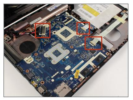
Locate the two strips and the wire bundle that are connected to the motherboard from other components.
