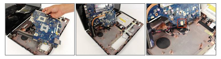
• Lift the motherboard carefully, and locate the last wire bundle that needs to be removed.
