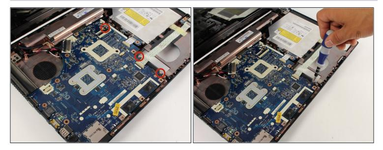
Now locate the three 1/4" diameter head and 7/32" length screws shown in the picture, and remove them with a #00 Phillips screwdriver.
