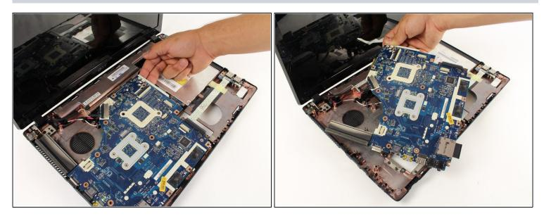
The motherboard should now be completely free of connections and easily removed.
