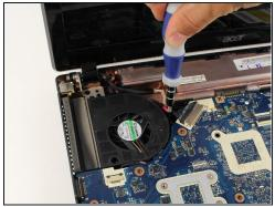
Once you manage to locate the fan use the screwdriver to unscrew the three screws highlighted.
