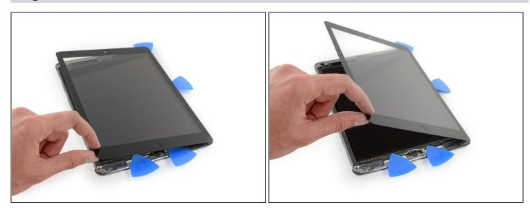
• Lift slowly and gently to further detach the adhesive along the display cable edge.
