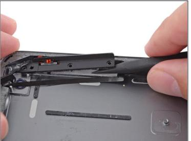
• Use the tip of a spudger to pry in the gap made by the opening pick, lifting the bracket off of the adhesive.
