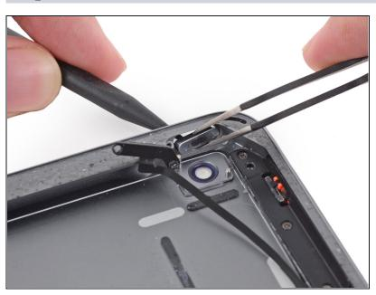
Push the power button into the case and remove it from the iPad.
