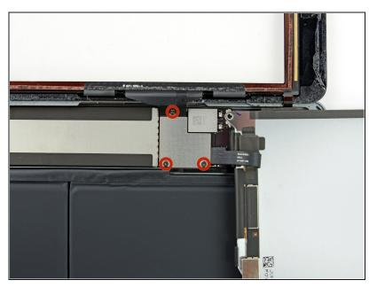
Remove the three 1.4 mm Phillips screws from the display cable bracket.
