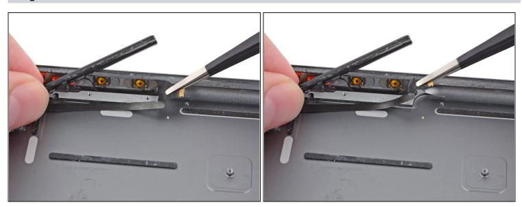
• Gently lift the connector end of the cable slightly off the rear case.
