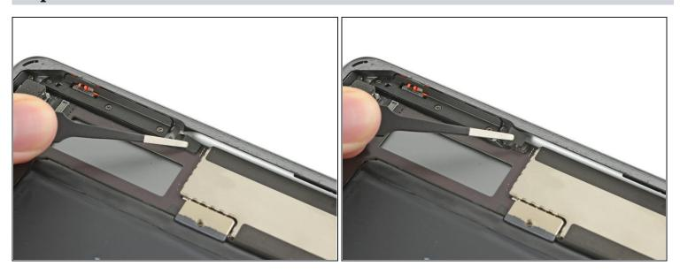
• Remove any tape covering the upper button assembly cable connector.
