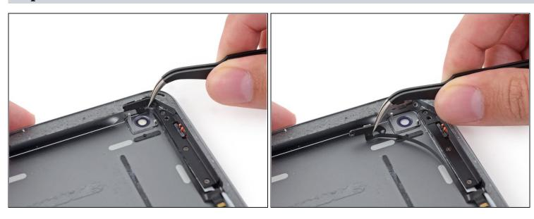
• With the power button cable bracket loosened, peel it off of the rear case with a set of tweezers and move it out of the way.
