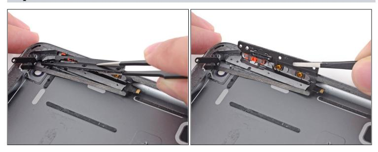
• With a set of tweezers flip the front end of the button bracket up to allow access to the rest of the button ribbon cable.
