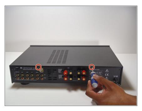
Remove 2 screws on rear of device.
