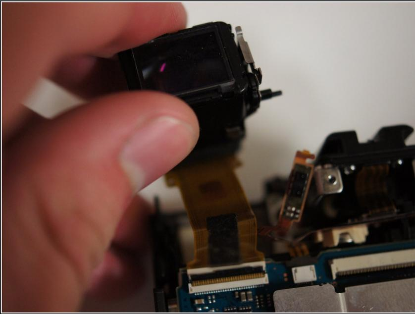
**⚠** Be gentle when removing the viewfinder because there is an orange ribbon cable connected to the body.
