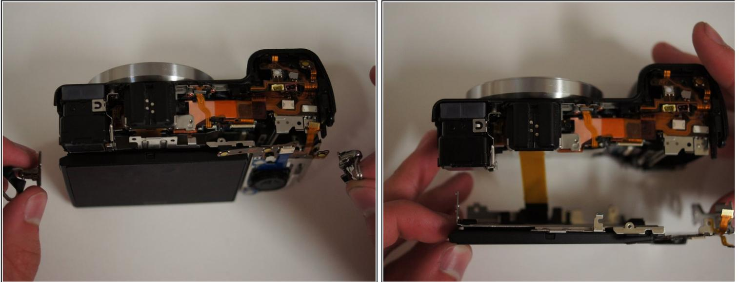
**⚠** The LCD assembly is attached with a concealed ribbon cable, so be gentle when you remove it.
