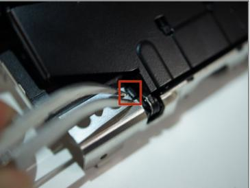
• Use the <u>tweezers</u> to push the tab near the bottom left corner of the panel to release a plastic cover from the back of the panel.
