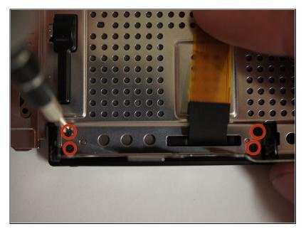
Remove the four 2/32" #00 screws from the metal bracket using the Phillips #00 screwdriver.
