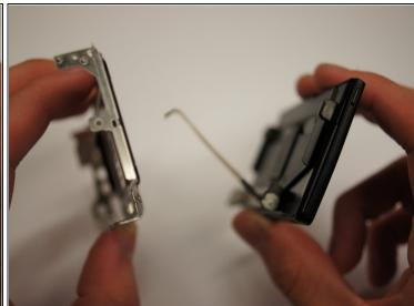
• Remove the screen from the metal panel.
