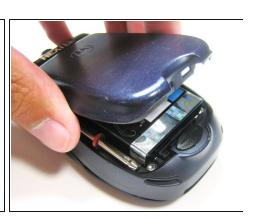
• Slide the notch downward while pulling the back cover off to remove it.
