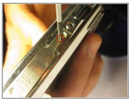
Using a #00 Philips Head Screwdriver, remove the screws located on all four sides of the camera.
