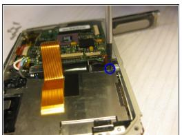
Unscrew four 2mm long screws using the #00 Phillips screwdriver.
