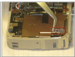
Remove four metal tabs from corners where the 2mm long screws were attached using tweezers.
