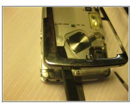
After removing all four of the screws, pry the side covers off of the camera.
