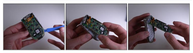
• Carefully pry and lift up on the logic board using an iPod Opening Tool.
