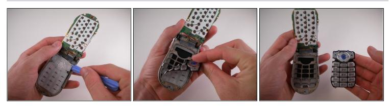
• Use an iPod Opening Tool to lift up on the keypad and pull it out.
