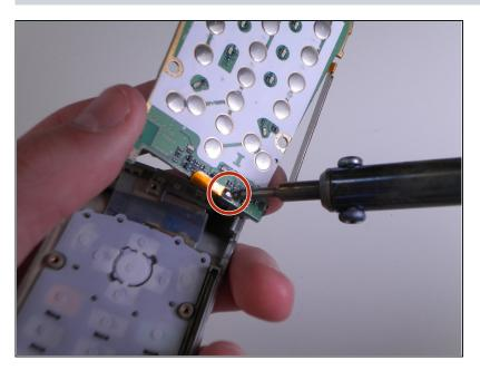
• Desolder the joint on the back using a soldering iron.
