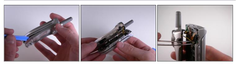
$\triangle$  When removing back cover, be careful not to break the speaker wires.
