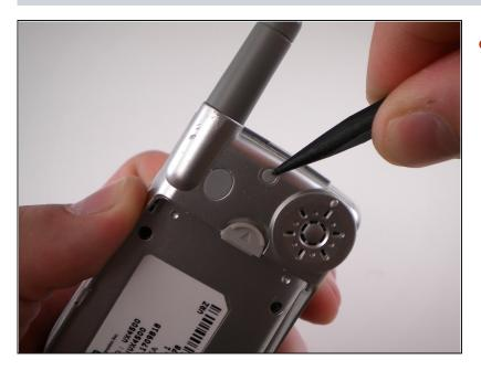
• Remove the rubber grommet using a Spudger.
