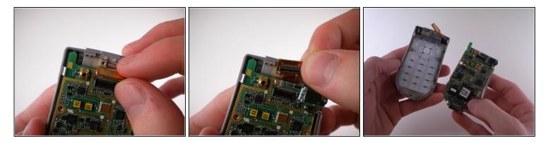
• Carefully detach the ribbon cable and remove the motherboard.
