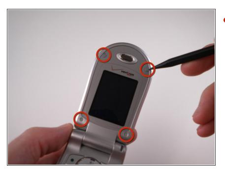
Remove 4 rubber grommets using the Spudger.
