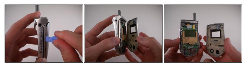
• Carefully pry off outer cover using iPod Opening Tool.
