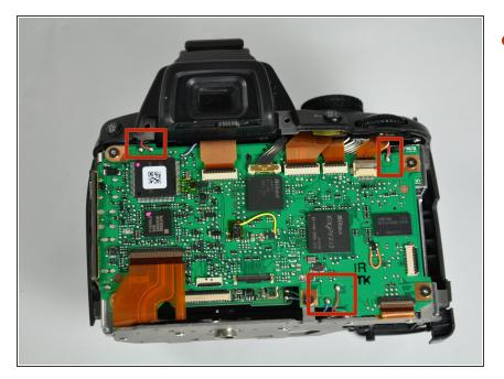
Desolder the five wires attached to the back of the board.
