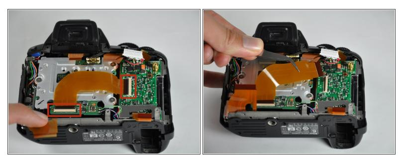
• Remove the L-shaped ribbon cable from both of its connectors.
