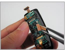
Disconnect the ribbon cables connecting the screen to the motherboard by lifting their metal connectors up off of the board with tweezers.
