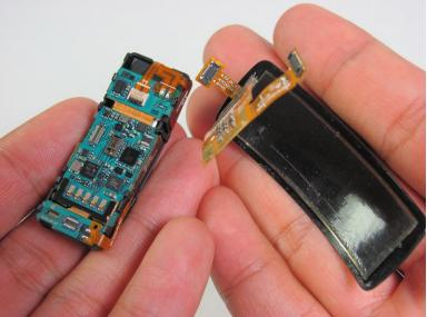
Gently peel the screen assembly up and away from the device using tweezers.
