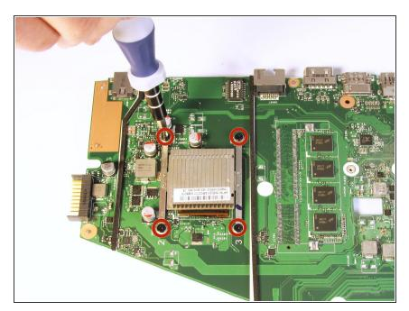
Remove the four 3.2 mm Phillips #0 screws holding the heat sink in place using the Phillips #0 Screwdriver.
