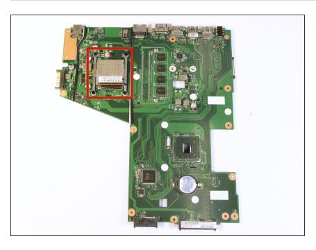
Flip the motherboard over and locate the heat sink.
