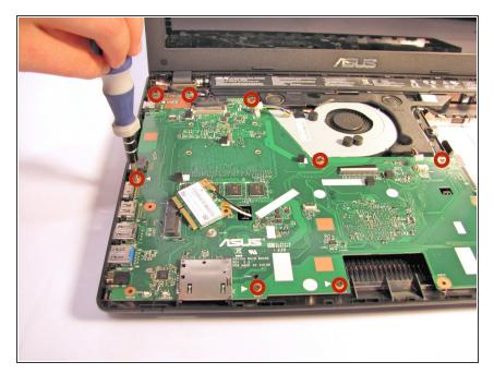
With the Phillips #0 Screwdriver, remove the nine 5.5 mm Phillips #0 screws which hold the motherboard in place.
