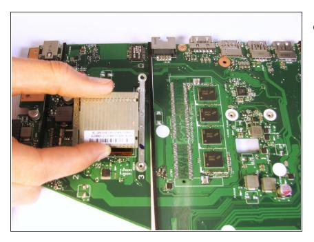
Finally, remove the heat sink by lifting it off the motherboard.
