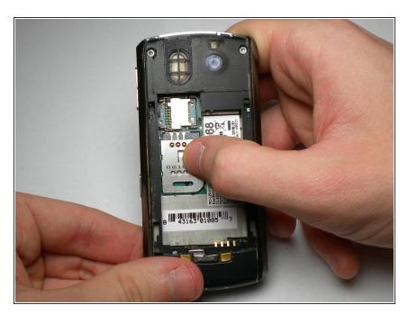
Slide the larger of the two metal casings upward (in the direction pointed to as "unlock").
