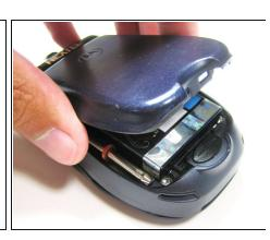
Slide the notch downward while pulling the back cover off to remove it.
