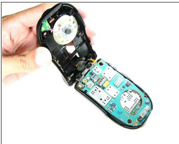
⚠ DO NOT force the cover off as it could damage the ribbon cable!
