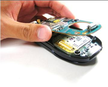
• Lift the first logic board off of the rest of the device.
