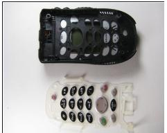
• Remove the keypad buttons off the front cover of the phone.
