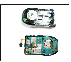
Carefully pry off the connection between the headphone jack and logic board.
