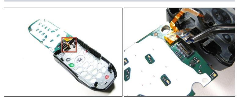
Using tweezers, carefully pull off the connector shown.
