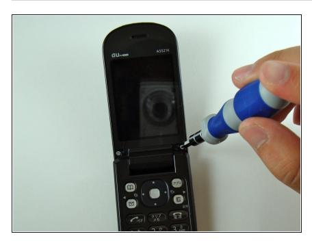
Remove the screws using a Y0 screwdriver.
