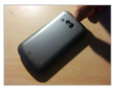
• First, remove the backplate by pushing the button at the top of the back of the phone.
