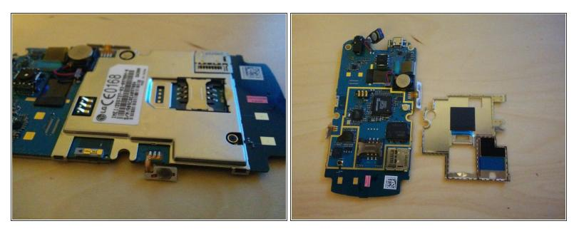
• The EMI shield can be removed by unclipping the clips on the side of the device.
