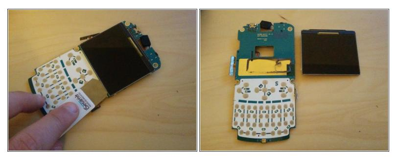
• Use a thin opening tool to separate the LCD from the main board.
