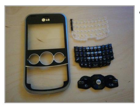
• The buttons on the front housing can then be pushed out through the back of the housing.
