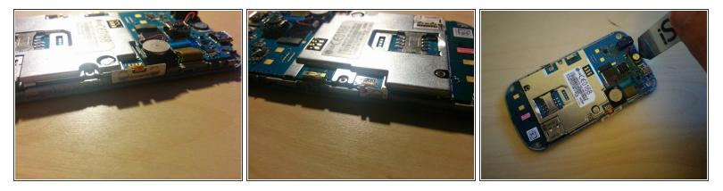
Both of these buttons need to be pried from the front casing to allow the mainboard to come away from the front housing.
