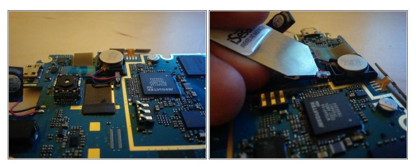
In the centre of the picture is the vibration module. It can be unclipped to remove it.
