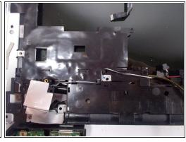
Remove wires from their grooves in casing.
