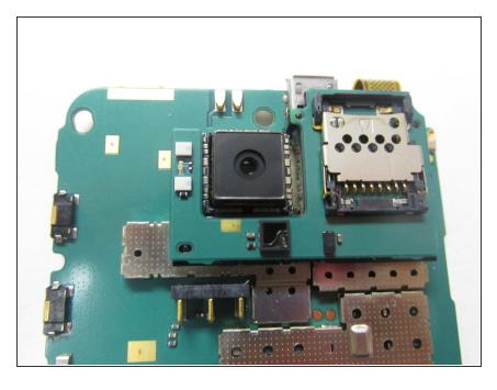
• The camera can be popped out easily using a blunt knife or credit card to pop it out. A new camera unit can be then simply put into the same place. In case a Nokia N900 camera unit cannot be found, it is possible to use a Nokia N79 camera without any ill effects. To reassemble your device, follow these instructions in reverse order.
